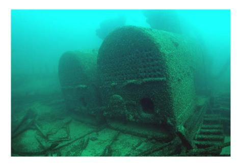
Figure 72. The *Selah Chamberlain*'s twin boilers are still attached to the steeple compound engine. Tamara Thomsen.
