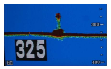
Figure 74. Sonar image of the *Tennie and Laura* showing the standing masts and rigging. Wisconsin Historical Society.
