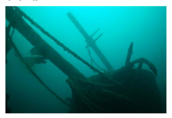
Figure 60. The *Gallinipper*'s bow, with bow knee, bowsprit, anchor, and mast. Tamara Thomsen.
