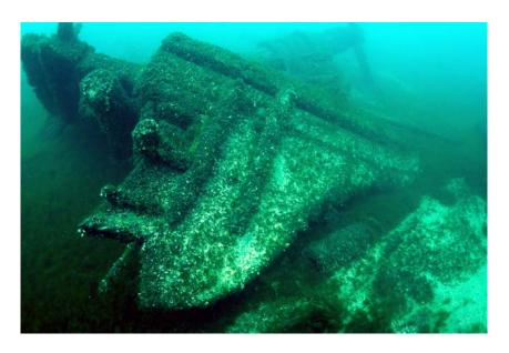
Figure 65. The *Mahoning*'s bow knee. The windlass is visible aft of the stem. Tamara Thomsen.
